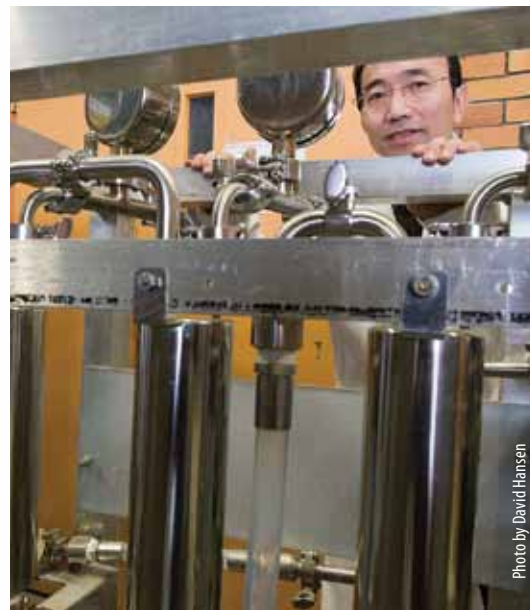
Left: A temperature map of ohmically heated whey and liquid produced by MRI imaging. Below: Roger Ruan poses with a prototype of a Concentrated High Intensity Electric Field (CHIEF) reactor that can more effectively and cost-efficiently destroy pathogens in food without altering its essential characteristics.
